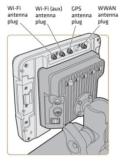
Because system performance and antenna polarization are site-dependent, a permanent mounting location may require some experimentation. In most fixed installations, you should mount the antenna initially in a vertically-polarized position, with the cable from the antenna parallel to the floor and ceiling. For information on purchasing an antenna, contact your local Intermec sales representative.
