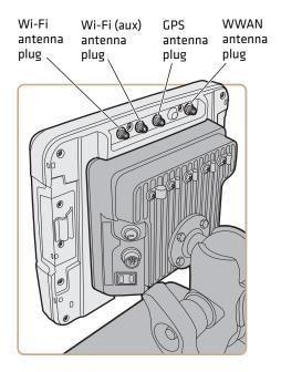
**3** Unscrew the antenna clamp on the smart dock and route the antenna wire through the antenna clamp.
