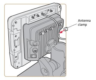
**4** Screw the antenna clamp back into the smart dock.
