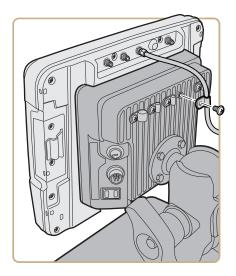
Because system performance and antenna polarization are site-dependent, a permanent mounting location may require some experimentation. In most fixed installations, you should mount the antenna initially in a vertically-polarized position, with the cable from the antenna parallel to the floor and ceiling. For information on purchasing an antenna, contact your local Intermec sales representative.
