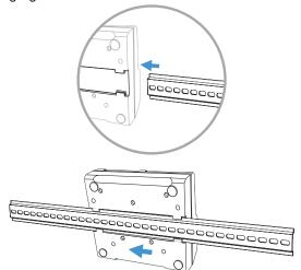
2. Using the appropriate hardware above, secure the DIN rail to the charge rack.
