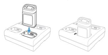
It is important that scanners are inserted into the charging pocket correctly. Inserting the scanner incorrectly could result in damage to the scanner or the charger.
