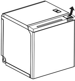
2. Install the roll paper in the correct direction of the roll paper.
