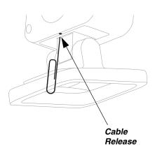
6. Replace with the new cable. Insert the connector into the opening and press firmly. The connector is keyed to go in only one way, and will click into place.
