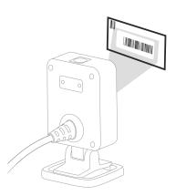
The aiming dot should be centered over the barcode, but it can be positioned in any direction for a good read. The aiming dot is smaller when the scanner is closer to the code and larger when it is farther from the code. Symbologies with smaller bars or elements (mil size) should be read closer to the unit. Symbologies with larger bars or elements (mil size) should be read farther from the unit.
