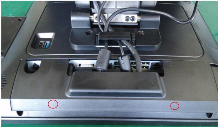
Step5: Assemble the base shell and tighten the tool-less screw;
