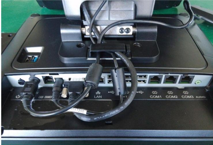
Step4: Assemble the cable shell, push the position of the red dot with thumb ;
