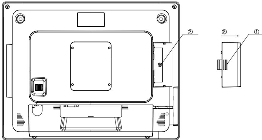
Step4: Pull the HD handle and remove the HD.
