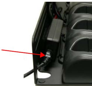
2. Plug the power supply into the correct outlet.
