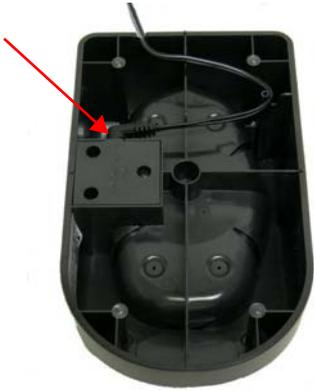
2. Guide the power supply cord through the slots to form a strain relief, as shown above.
