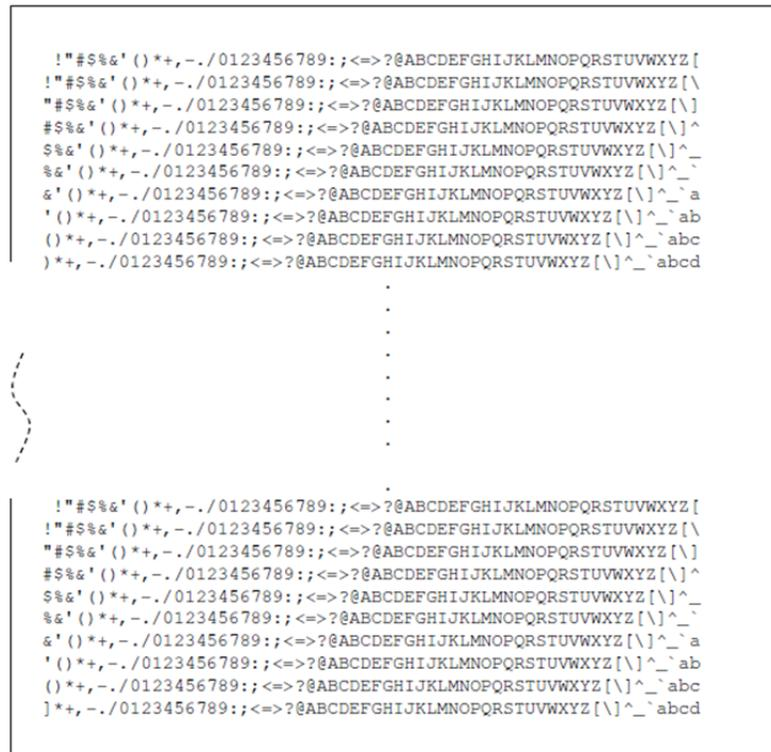
To pause the printing test, press **READY/CLEAR**. Press **READY/CLEAR** again to resume the printing test.
