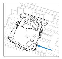
**3** Squeeze the tabs on the sides of the ribbon cartridge and lift the cartridge out of the printhead.
