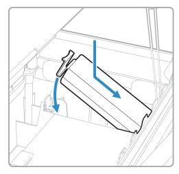
4 Press the battery down into the bay until it snaps into place.
