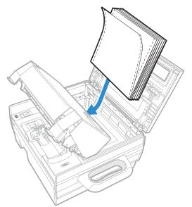
**3** Carefully tilt the printer mechanism back into the case. The first sheet of paper should be threaded between the back of the mechanism and the printer case.
