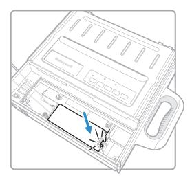
6 Press the battery clip into the clip holder.
