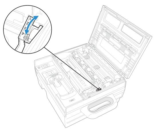
1 Verify the type and thickness of paper you are using. Look in "Recommended Printhead Gap Settings" for your paper type, and set the green printhead gap lever to the recommended setting.
