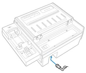
*Power port location (Fixed mount printer, portable printer with 200-sheet paper tray)*
