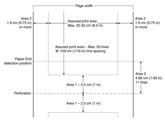
You should leave a 1 inch margin at both the top and the bottom of the page. This provides for a margin of six lines at 1/6 inch line spacing. Even though printing in Area 1 (before or after the perforation) may be possible, you should keep in mind that paper feed precision is reliable only within the Assured Print Area.
