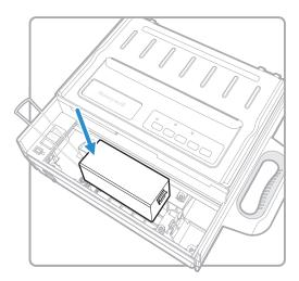
**5** Press the battery down into the bay until it snaps into place.
