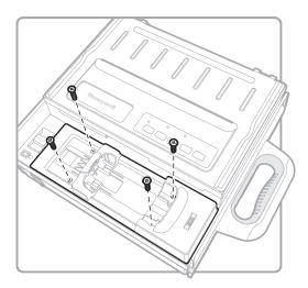
**2** Lift the computer holder out of the printer case. Be careful not to disconnect the wiring.
