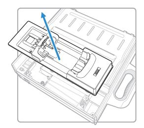
**3** Squeeze the battery clip and lift it away from the battery bay.
