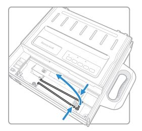
**4** Insert the battery into the bay, contact end first. Make sure the contacts are on the bottom, facing the side closest to the wiring.
