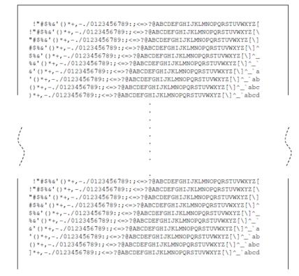
To pause the printing test, press **READY/CLEAR**. Press **READY/CLEAR** again to resume the printing test.
