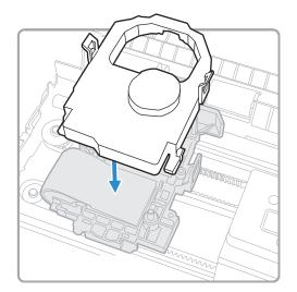
7 Release the tabs and gently rock the cartridge from side to side to make sure the tabs are seated in the clamps.
