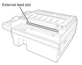
External media feed slot (Fixed mount printer)
