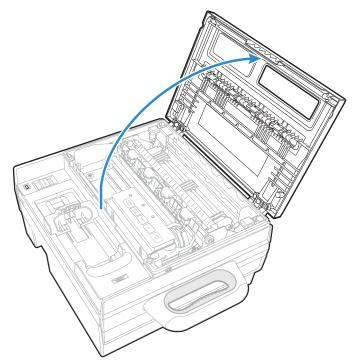
2 If necessary, slide the printhead out from behind the control panel.
