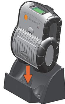
**Note:** Make sure you regularly clean the charging contact points on your printer's case to ensure your printer's batteries are properly charged, and to avoid damage to the printer or the charger. To clean the charging contact points, use alcohol and a clean rag.
