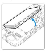
$7. \ \ \, \text{Lift up the edge of the SD card access door.}$
