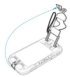
3. Press and hold down the small button on the battery latch, and then slide the latch toward the bottom of the computer to unlock the battery.
