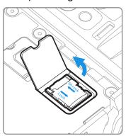
8. Press down gently and slide the card holder toward the open access door. Lift the edge of the holder up.
