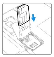
10. Close the holder with the card installed. Press down gently on the holder and slide it into the locked position.
