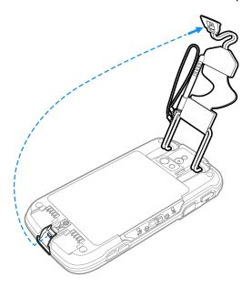
5. Press and hold down the small button on the battery latch, and then slide the latch toward the bottom of the computer to unlock the battery.
