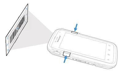
4. Release the Scan button when the computer beeps, and the Good Read LED briefly turns on. The barcode information is entered into the application in use.
