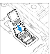
10. Close the holder with the card inserted. Press down gently on the card holder and slide it into the locked position.
