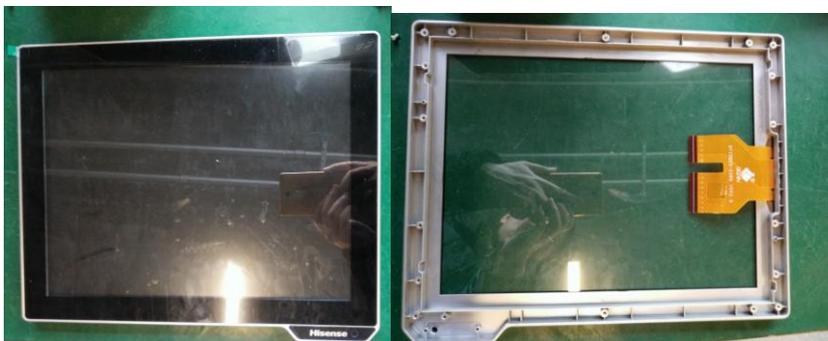
**Notes:** touch panel is pasted to front shell by 3M tape tightly, so it is hard to disassemble the touch screen and front shell, so we suggest you may replace front shell and touch panel assy to avoid part damage. The parts needed as below:
