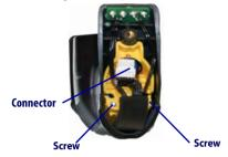
Carefully lift out the gold contacts circuit, and remove the battery holder cap while letting the white connector pass through the hole in the battery holder (as shown below).
