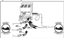
**Power Connection:** Plug the AC Adapter into an approved AC wall socket with the cable facing downwards (as shown in Figure 1) to prevent undue strain on the socket.
