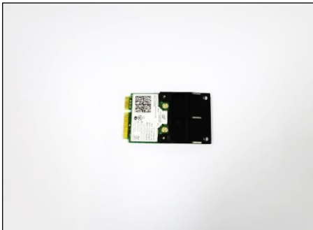
A Wi-Fi module and mini PCIe adapter assembly.
