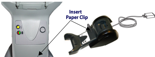
Figure 5. Disconnecting the Cable
