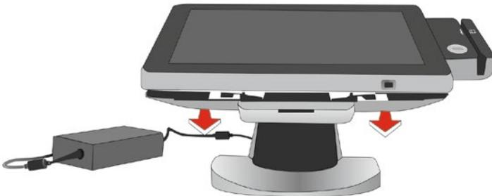
Remove the cover of the pedestal by pressing and thus releasing the locking (see arrow). Lift the cover out of the pedestal by lifting it upwards and slightly forwards.
