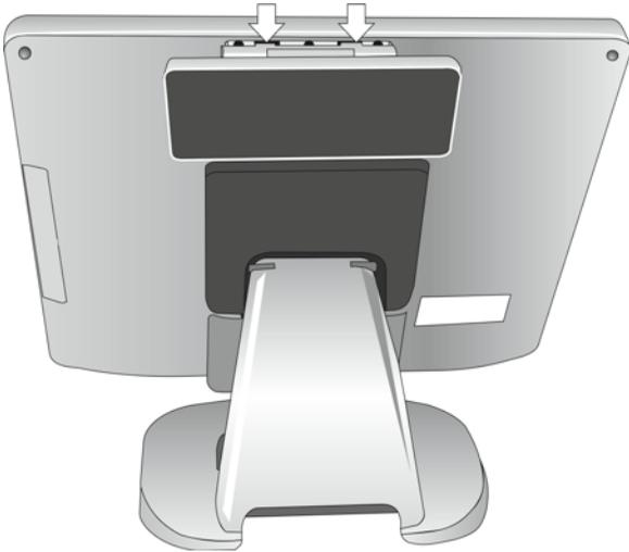
Flap the display upwards and tighten it with the delivered screws.
