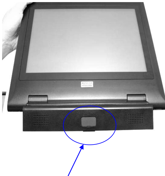
Location to install waiter lock
