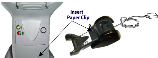
Figure 5. Disconnecting the Cable
