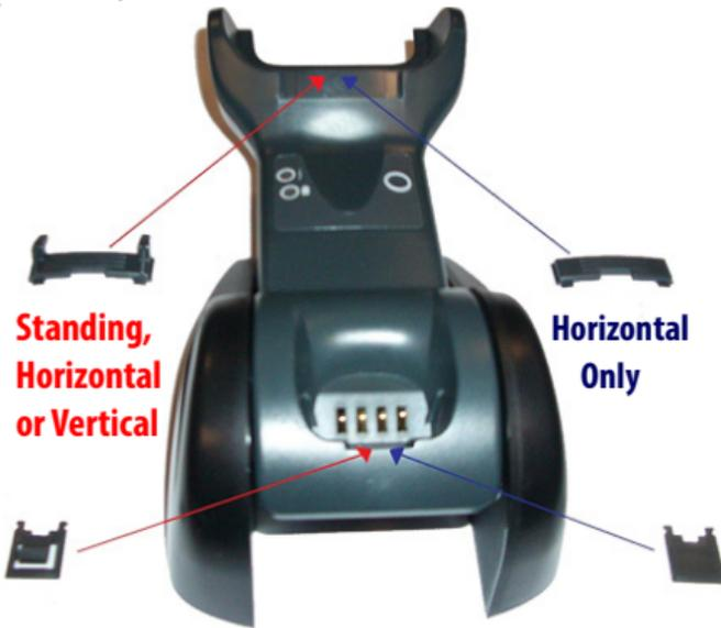
2. Using your thumbs, push open the plastic tabs on the bottom of the base to free the wing holders.
